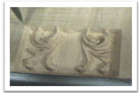
FIGURE I.6 RASTER CARVING LINE BY LINE
