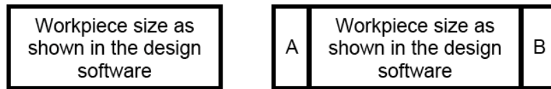
FIG 2.2.2 - 7 Inch Rule. A & B showing the extra 3 1/2 inches on both ends of the board
