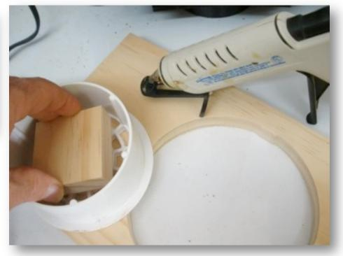
Insert two drain caps into the ends of the 3-inch pipe. The fit should be tight. Drill a 7/32-inch pilot hole in the wood
