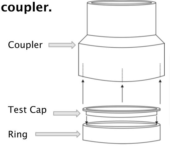
The fit should be snug. Secure from the inside with aluminum duct tape, if necessary.
